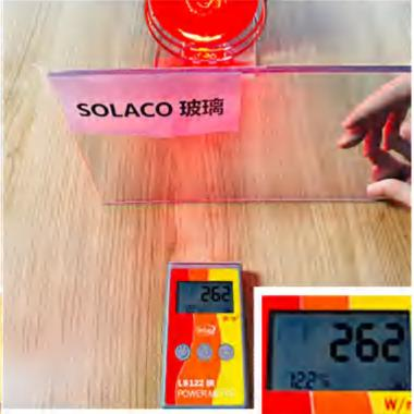
Under the same light source, SOLACO Auto grade heat insulation glass, the light intensity value is 262, the infrared rejection rate is 87.8%..
